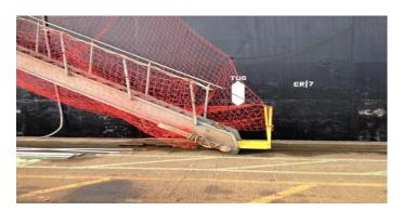
Safety netting rigged from ship's side, under the accommodation ladder and secured to outboard top rail
