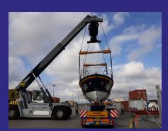
Max lifting capability: 45 tonnes
