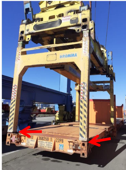
Fig. 2 Up part of corners casting available for lifting
