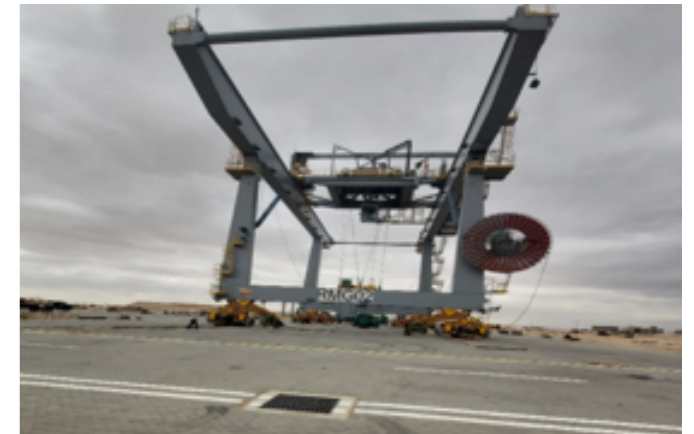
Offloading for two RMG and move it to the yard, commissioning started by ZPMC team
