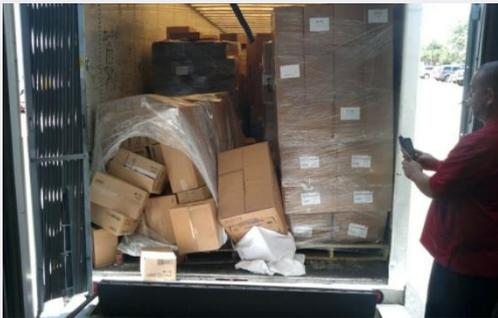
Figure 4.1 Lack of proper securing during movement
