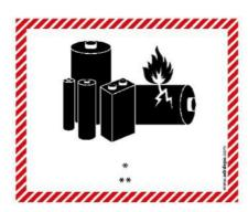
As per clause 188 packages including prepared lithium battery will be tagged with lithium battery tag. The tag will have "UN" letter which will be followed by the UN numbers,
