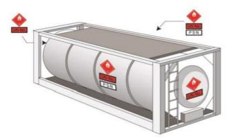
4 sides of the container should be tagged with warning signs which represents the class of the dangerous goods that it's transporting.
