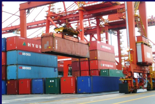
RTG (Rubber Tire Gantry)
